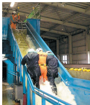
実物大階段模型（流水階段） Scale model of a staircase (Water inflowing staircase)
