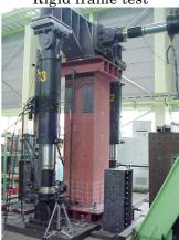
Steel bridge pier test
