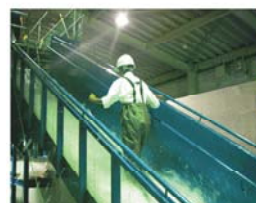
Figure 1. Experiments at the Ujigawa Open Laboratory of flood evacuations from underground facilities.
