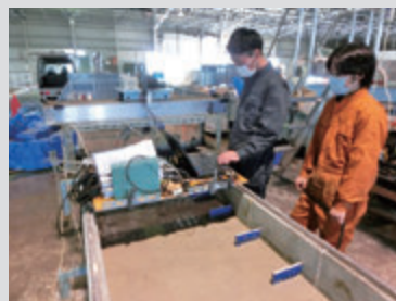
水制設置による河床変動実験 Experiment on riverbed variation caused by spur dyke installation
